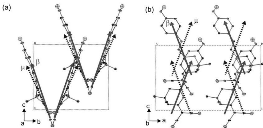
**Figure 5.** Crystal packing diagram of OH1 crystal projected along the  $a$ -axis (a) and along the  $b$ -axis (b). The solid and dotted vectors present the directions of the maximum first hyperpolarizability  $\beta_{max}$  and the dipole moment  $\mu$  of four OH1 molecules in the unit cell as determined by finite-field calculations, respectively. Hydrogen atoms excluding those on OH group are omitted for clarity.
