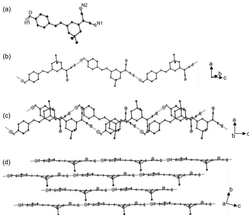
**Figure 3.** a) Molecular structure of the OH1 chromophore in the crystalline state. Acentric polymer-like chains: top view of an acentric chain (b), top (c), and side (d) view of a stack of acentric chains. Hydrogen atoms excluding those on OH group are omitted for clarity. OH1 molecules in the acentric chain are linked with hydrogen bonds of  $\text{C}\equiv\text{N}\cdots\text{H}-\text{O}$  with  $\text{N}\cdots\text{H}$  distances of about 2.12 Å, which are indicated by dotted lines.
