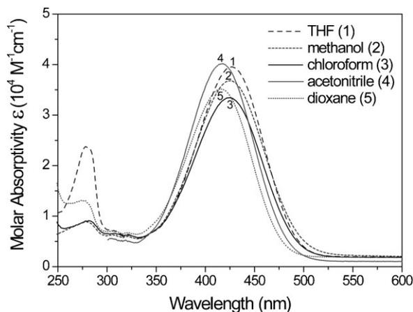
**Figure 1.** Absorption spectra of OH1 molecule in different solvents: THF (1,  $\lambda_{\text{max}} = 427$  nm), methanol (2,  $\lambda_{\text{max}} = 426$  nm), chloroform (3,  $\lambda_{\text{max}} = 423$  nm), acetonitrile (4,  $\lambda_{\text{max}} = 417$  nm), and dioxane (5,  $\lambda_{\text{max}} = 415$  nm).
