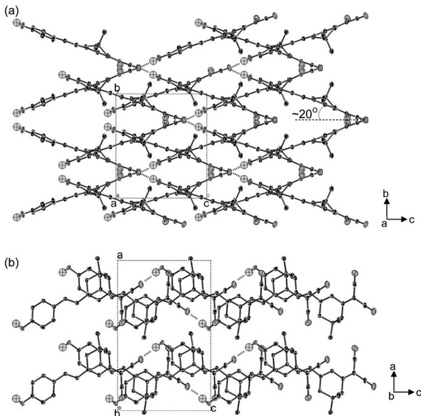
**Figure 4.** The relative arrangement of both acentric layers in OH1 projected along the  $a$ -axis (a) and along the  $b$ -axis (b). Hydrogen atoms excluding those on OH group are omitted for clarity.
