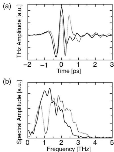
**Figure 7.** Few-cycle terahertz pulses generated in single crystals of OH1 (thickness 0.365 mm, solid line) and DAST (thickness 0.400 mm, dotted line) at a laser wavelength of 1460 nm. a) Time-domain waveforms of the terahertz electric field  $E(t)$ . b) Their frequency spectra  $E(\nu)$ .
