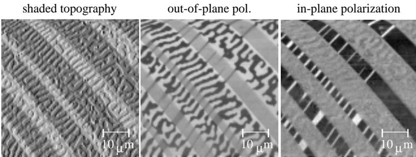
Fig. (a)  $\text{BaTiO}_3$  sample surface topography, and (b) and (c) the out-of-plane and in-plane component of the electric field at the sample surface, respectively.
