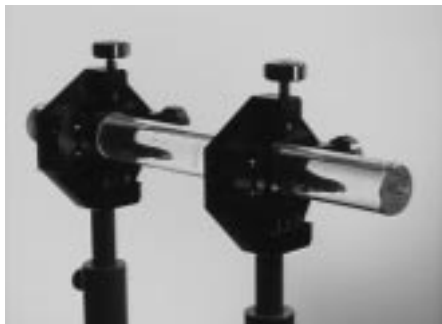
Liquid Stimulated Brillouin Scattering (SBS) cell for optical phase conjugation
