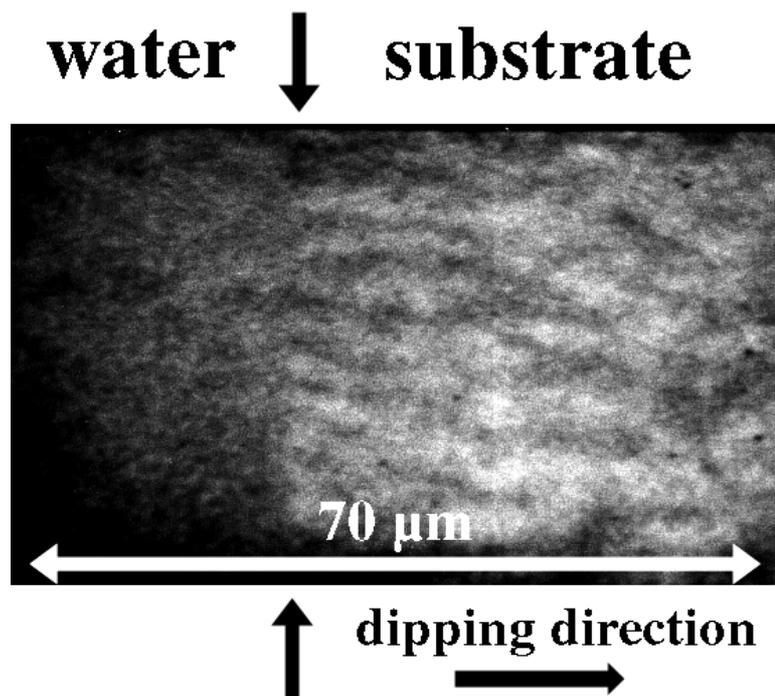
Fig. 1 Film transfer of LB molecules from water subphase (left) to the substrate (right) reorients the LB molecules parallel to the direction (see arrow)
